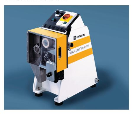
The Strand Pelletizer CSG 171 T is the universal equipment for granulating 1 to 3 strands. Precise speed control, wide range adjustment, exact cutter clearance together with visual access by means of a polycarbonat cover does make this unit to be the optimal tool for granulating small batches of 0,1 to 10 kg/h.
