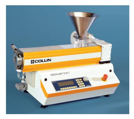
The single-screw extruder is the standard unit for the continuous plastification of polymers.
