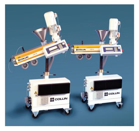
The extruder is a special design with separate electric cabinet.
